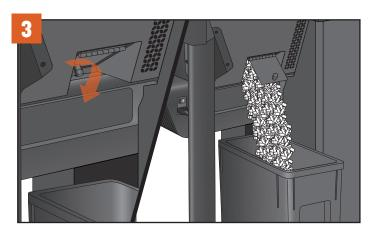
Unscrew the knob on the back of the auger box and open the pellet release door. Pellets will empty into the StayDry™ Pellet Bin. Vacuum out any remaining sawdust from the hopper and auger.
