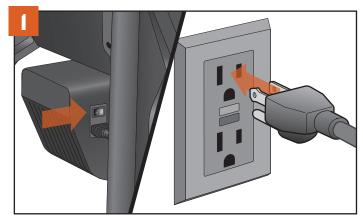
With the main power switch set to OFF (0), connect the power cord to your grill. Then plug the power cord into a properly grounded/earthed electrical outlet protected by a Ground Fault Circuit Interrupter (GFCI).
