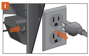
Press the main power switch to OFF (0) and disconnect the power cord. If the grill is still hot, allow it to cool completely.
