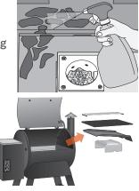
accumulation from inside the V-shaped grease drain and grease drain tube using a stiff, nonmetallic tool. Much of the loosened grease can be pushed down through the grease drain tube and will fall into the grease bucket. Wipe up remaining grease residue with paper towels or disposable rags. Regularly clean the grease out of the grill barrel on the interior bottom and sides. If grease is allowed to build up, a grease fire could result.
