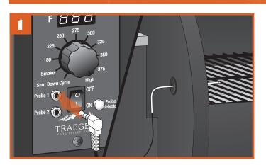
Insert I or 2 meat probes into the plug-in holes on the lower left corner of the controller; then thread probes through the access hole grommet on the left side of the grill barrel.
