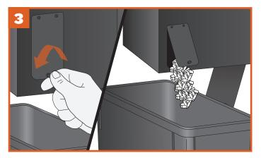
Unscrew the clean-out door fastener and open it. Pellets will empty into the Pellet Bin you've placed below. You might need a spatula or spoon to push the remaining pellets out of the hopper.
