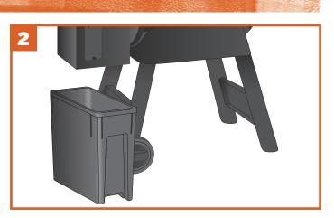
Place the Pellet Bin (purchased separately) to hold the unused pellets under the pellet hopper clean-out door.
