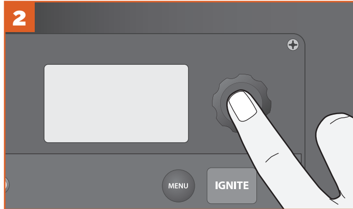
Press the center of the selection dial to wake the grill.
