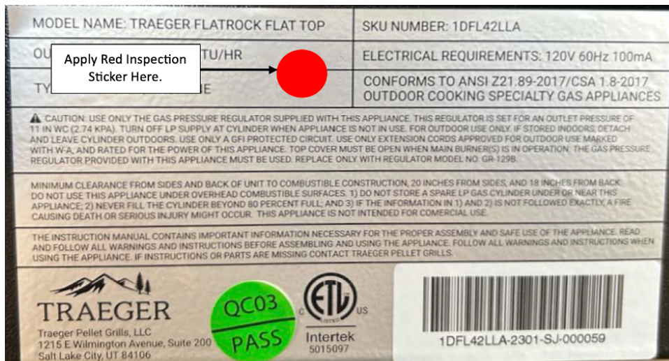
Figure 7. Placement of red inspection sticker on the Flatrock data plate label.
