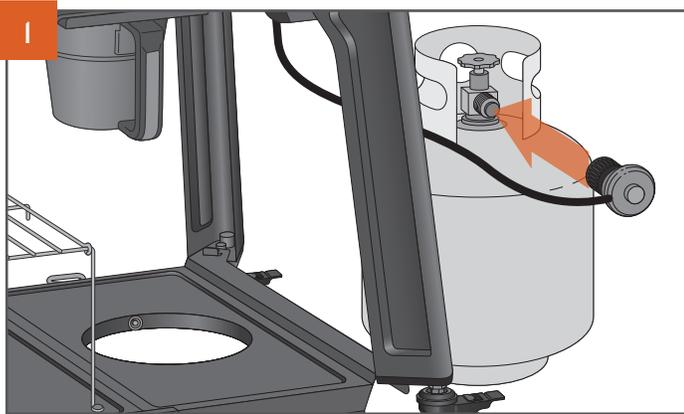
Be sure both control knobs are in the OFF (O) position. Screw the end of the regulator onto the propane tank valve. Hand-tighten.
