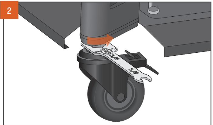
Tighten jam nut all the way with included wrench to lock leveling. The jam nut is underneath the leg but above the caster.
