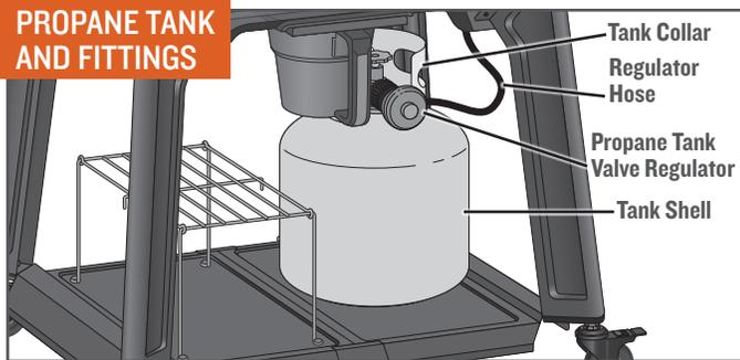
The Flat Top Grill can be used with any standard 20 lb (9 kg) propane tank. It must be a maximum of 12 1/4" in diameter; 18" high, and with right-handed connection threads. The tank must be marked in accordance with the latest U.S. Department of Transportation specifications for LP gas tanks or DOT. CFR49 or National Standards of Canada CAN/CSA-B359 Cylinders, Spheres and Tubes for the
