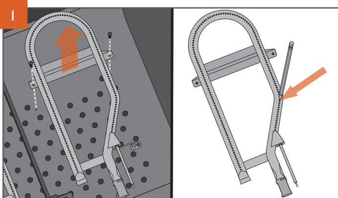
Remove burners from the Flat Top Grill by unscrewing the two fasteners on the burner brackets. With burner removed, insert a pen tip or paperclip into the clogged burner inlet hole to clear out any debris that may have accumulated.
