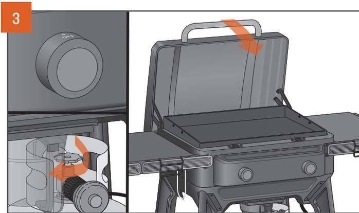
Turn both control knobs to the OFF (O) position, close the lid, and turn the propane tank valve closed. Always shut off the propane tank valve completely after every cook.
