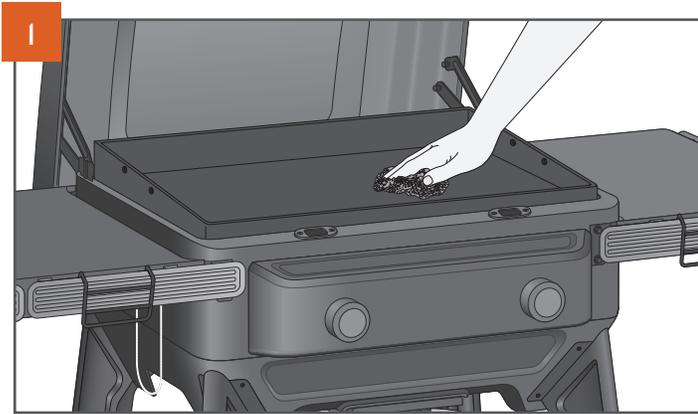
Use a nonabrasive scouring pad and water to remove rust. If rust cannot be removed with the nonabrasive scouring pad, you can use 220 grit sandpaper to remove rust from affected areas.
