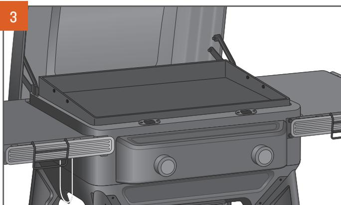
Preheat the Flat Top Grill on high for 10 minutes. Make sure the propane tank valve has been turned to the fully open position. Press the control knob and rotate to the ignite position (🔥). Turning the knob opens the control valve and activates the igniter. Look at
