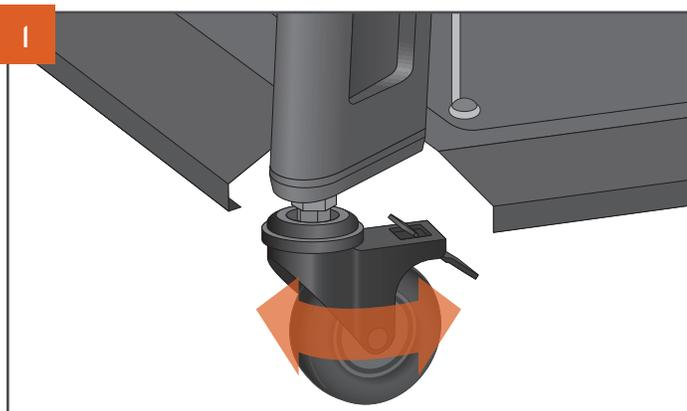
Level grill by adjusting the position of each caster individually. To adjust caster position, set the caster lock and rotate the caster by hand. Adjusting to the right will shorten the position, and to the left will extend it. Once you've got your desired level, proceed to step 2.
