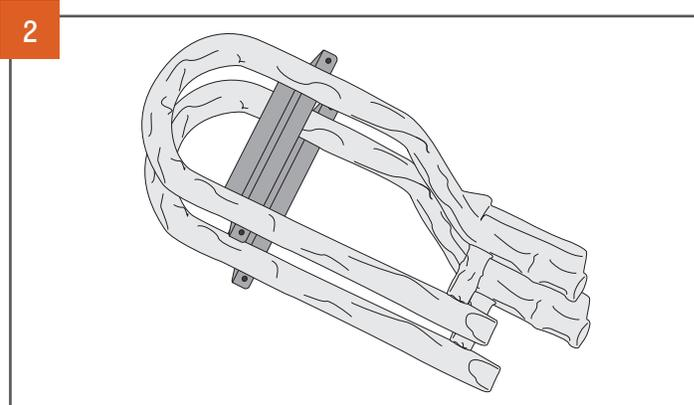
When storing the Flat Top Grill or before an extended period of non-use, remove the burners and wrap them with aluminum foil to reduce the risk of insects entering the burner holes.
