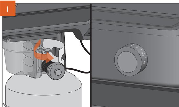
Make sure the propane tank valve has been turned to the fully open position. Press the control knob and rotate to the ignite position (🔥). Turning the knob opens the control valve and activates the igniter. Look at the burner through the flame window to confirm that the burner has successfully lit. If the burner did not light, turn the control knob back to the OFF (○) position and repeat until burner ignition is confirmed.
