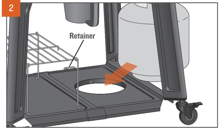
With the regulator connected to the tank, place the tank in the opening in the bottom shelf. Secure the tank in place by hand-tightening the tank retainer.
