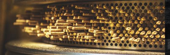
2 The sawdust is compressed into pellets using heat and pressure.
