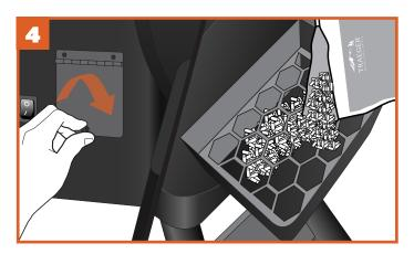
Once the hopper is empty, close the clean-out door, replace the fastener, and refill the hopper with your preferred flavor of TRAEGER® BRAND HARDWOOD PELLETS.
