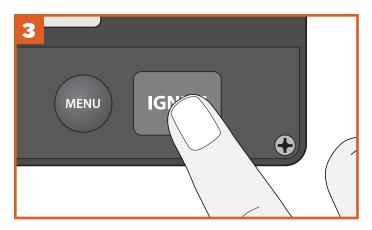
Press IGNITE to begin the automatic ignition and preheat cycle.
