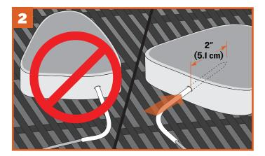
Insert the probe tip into the thickest part of the meat—not in the fatty portion or touching bone. The probe needs to be in the meat at least 2" (5.1 cm). This probe may not be suitable if you can't insert the probe into the thickest part of the meat and 2" (5.1 cm) into the meat.
