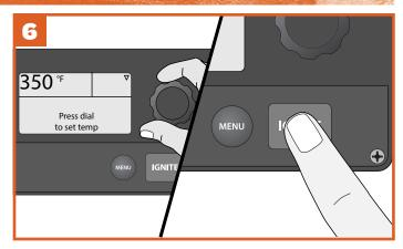
The home screen will display "Press dial to set temp." Turn the selection dial clockwise to 350°F (I75°C) and press the dial. Next, close grill door, press IGNITE, and run grill for 20 minutes after it reaches 350°F (I75°C).
