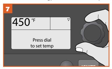
Adjust temperature to 450°F (232°C) and run grill for an additional 30 minutes after it reaches 450°F (232°C).
