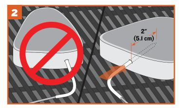
Insert the probe tip into the thickest part of the meat—not in the fatty portion or touching bone. The probe needs to be in the meat at least 2" (5.1 cm). This probe may not be suitable if you can't insert the probe into the thickest part of the meat and 2" (5.1 cm) into the meat.
