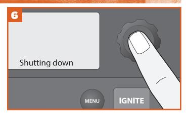
Turn off the grill by pressing and holding the selection dial for 3 seconds, initiating the shut-down cycle.
