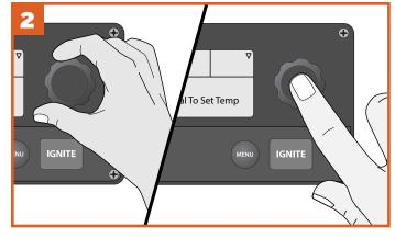
To select temperature, turn selection dial right or left; once desired temperature is displayed, press the center of the dial to select. Close the grill door.
