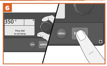
The home screen will display "Press dial to set temp." Turn the selection dial clockwise to I75°C (350°F) and press the dial. Next, close grill door, press IGNITE, and run grill for 20 minutes after it reaches I75°C (350°F).
