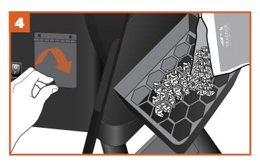
Once the hopper is empty, close the clean-out door, replace the fastener, and refill the hopper with your preferred flavor of TRAEGER BRAND HARDWOOD PELLETS.
