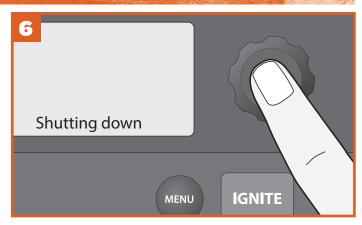
Turn off the grill by pressing and holding the selection dial for 3 seconds, initiating the shut-down cycle.
