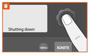
Turn off the grill by pressing and holding the selection dial for 3 seconds, initiating the shut-down cycle. When the full shut-down cycle finishes, seasoning of your grill is complete.
