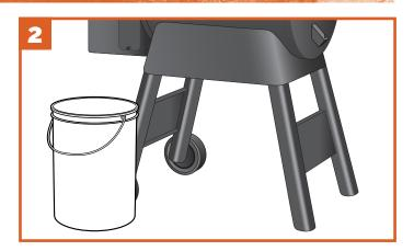
Place a container large enough to hold the unused pellets under the pellet hopper clean-out door.
