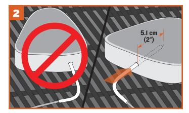
Insert the probe tip into the thickest part of the meat—not in the fatty portion or touching bone. The probe needs to be in the meat at least 5.1 cm (2"). This probe may not be suitable if you can't insert the probe into the thickest part of the meat and 5.1 cm (2") into the meat.
