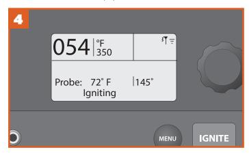
Once the probe alarm is set, the home screen will display the grill temperature, goal probe temperature, and grill status. A tone will sound when your meat reaches the set alarm temperature. If using the Traeger app, you can monitor the probe temperature, you can adjust the probe temperature, and you will receive a push notification on your connected smart device when the desired temperature is reached.
