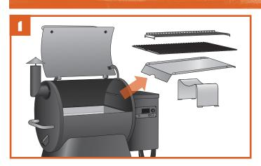
Remove the porcelain-coated grill grates, grease drip tray, and heat baffle from the inside of the grill.
