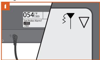
Plug the probe into the probe jack located on the WiFIRE Controller. The controller will recognize the probe and the probe icon will light in the controller screen's upper-right corner. The display will ask if you want to set an alarm. Select YES.
