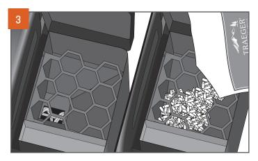
Open the hopper lid. Make sure there are no foreign objects in the auger before adding pellets to the hopper. After adding pellets to the hopper, close the hopper lid. We recommend you fill the hopper with pellets at least to the safety grate in the hopper.
