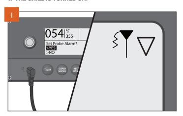
Plug the probe into the probe jack located on the WiFIRE® Controller. The controller will recognize the probe and the probe icon will light in the controller screen's upper-right corner. The display will ask if you want to set an alarm. Select YES.
