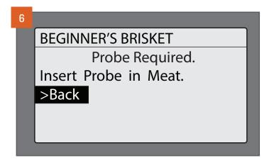
If the probe is required, you'll be instructed to insert the probe into your meat (see "Cooking with the Meat Probe" section on page 24). After you have followed the probe insertion instructions, a tone will sound once to indicate that the probe is recognized. To RUN COOK CYCLE NOW, select YES at the prompt.
