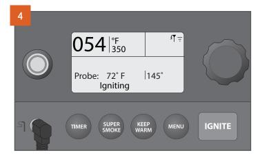
Once the probe alarm is set, the home screen will display the grill temperature, goal probe temperature, and grill status. A tone will sound when your meat reaches the set alarm temperature. If using the Traeger app, you can monitor the probe temperature and adjust the probe temperature, and you will receive a push notification on your connected smart device when the desired temperature is reached.
