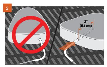
Insert the probe tip into the thickest part of the meat—not in the fatty portion or touching bone. The probe needs to be in the meat at least 2 inches (5.1 cm). This probe may not be suitable if you can't insert the probe into the thickest part of the meat and 2 inches (5.1 cm) into the meat.
