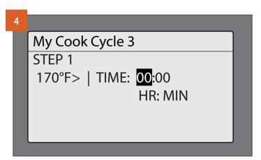
If the recipe calls for a specific number of hours at a set temperature, select TIME. To select hours, rotate the dial. Press to select and move to minutes. Rotate to choose minutes and press the dial to select.
