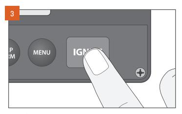
Press IGNITE to begin the automatic ignition and preheat cycle.
