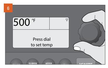
Adjust temperature to 500°F (260°C) and run grill for an additional 30 minutes after it reaches 500°F (260°C).
