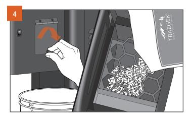
Once the hopper is empty, close the clean-out door, replace the fastener, and refill the hopper with a different flavor of TRAEGER® ALL-NATURAL HARDWOOD PELLETS.
