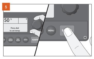
The home screen will display "Press dial to set temp." Turn the selection dial clockwise to  $350^{\circ}F$  (175°C) and press the dial. Next, close grill door, press IGNITE, and run grill for 20 minutes once it has reached  $350^{\circ}F$  (175°C).
