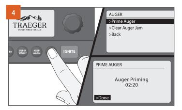
Turn grill on: Flip the main power switch on the back of the grill to ON (I); then press the Standby button to wake the grill. Press MENU to display the main menu. Turn the dial to select AUGER; then select Prime Auger.
