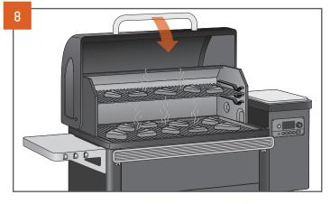
The automatic ignition and preheat cycle will begin. Once preheating is complete, load food into the grill. See page 24 if using the meat probe prior to loading food into the grill. Close the grill door to proceed with your custom cook cycle. Unlike a gas grill, you must keep the grill door shut during cooking.
