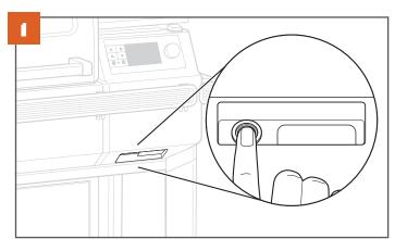
Press the main power button located on the front of the grill to **ON**.
