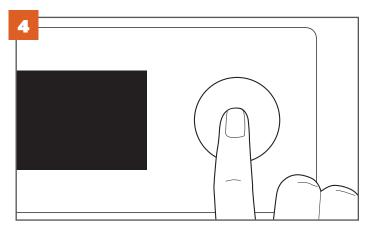
To shut down the grill, press and hold the selection dial for 3 seconds.
