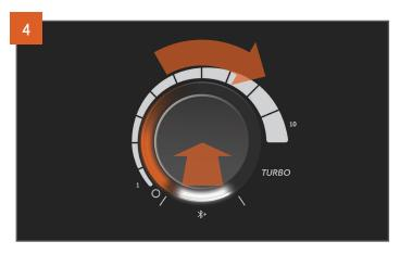
To change power level, simply turn the control dial to a new power level and press the dial to confirm the selection.
