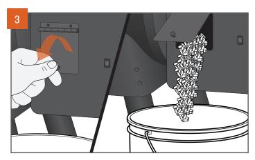
Unscrew the clean-out door fastener and open it. Pellets will empty into the container you've placed below. You might need a spatula or spoon to push the remaining pellets out of the hopper.
