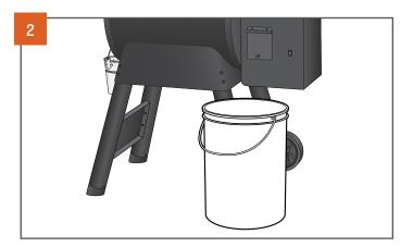
Place a container large enough to hold the unused pellets under the pellet clean-out door.
