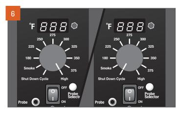
Turn the temperature dial to HIGH. Once pellets begin to fall into the firepot, the auger is primed. Turn the dial to SHUT DOWN CYCLE to reset the ignition process.
