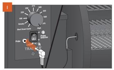
Insert the meat probe into the plug-in hole on the lower left corner of the controller; then thread probe through the access hole grommet on the left side of the grill barrel.
