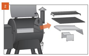
Open the door and remove all food, the porcelain-coated grill grates, the grease drip tray, and the heat baffle.
