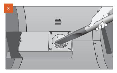
WARNING! AFTER THE GRILL, PELLETS, AND ASH HAVE COMPLETELY COOLED, REMOVE ALL UNBURNED PELLETS AND ASH FROM INSIDE AND AROUND THE FIREPOT. (SEE INSTRUCTIONS FOR PROPER HANDLING AND DISPOSAL OF ASH ON PAGE 23.)
