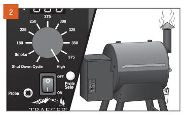
Turn the temperature dial to your desired temperature. After two minutes, pellets will begin to ignite and whitish-gray smoke will come out of the grill. For best results, allow the grill to preheat for 10 minutes with the door closed before placing food in the grill.
