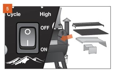
When flames start to come out of the firepot, turn the main power switch OFF (0). Let the grill completely cool. Place the heat baffle, grease drip tray, grill grates, and food back into the grill.
