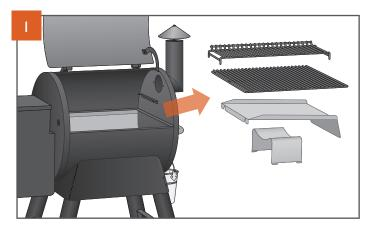
Remove the grill grates, grease drip tray, and heat baffle from the inside of the grill.
