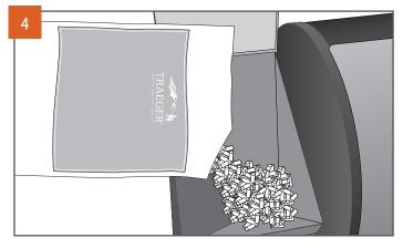
Open the hopper lid. Make sure there are no foreign objects in the auger before adding pellets to the hopper. After adding pellets to the hopper, close the hopper lid. We recommend you fill the hopper with pellets at least to the safety grate in the hopper.
