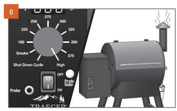
Turn the main power switch ON (I). Turn the temperature dial to your desired temperature. After two minutes, pellets will begin to ignite and whitish-gray smoke will come out of the grill. For best results, allow the grill to preheat for IO minutes with the door closed before placing food in the grill.
