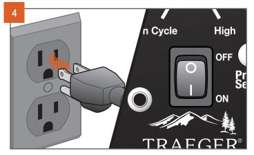
Plug power cord into an appropriate grounded electrical outlet and restart the grill. Pellets should fall into the firepot and the hot rod should begin to heat (it will start to turn red).
