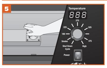
Check that there is air movement from the draft inducer fan by placing your fingers over the firepot.
