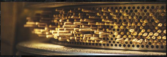
2 The sawdust is compressed into pellets using heat and pressure.
