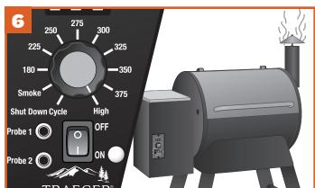
Turn the temperature dial to your desired temperature. After two minutes pellets will begin to ignite and whitishgray smoke will come out of the grill. For best results, allow the grill to preheat for IO minutes with the door closed before placing food in the grill.
