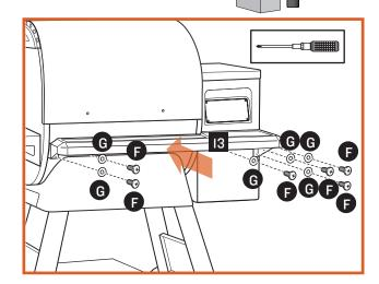
**INSTALL HANDLE AND GREASE PAN WITH LINER**
