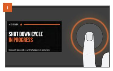
Press and hold the selection dial down for 3 seconds, until the screen registers and shows "SHUT DOWN CYCLE IN PROGRESS."
