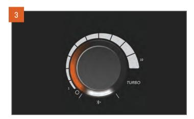
After pressing the control dial to select power level, the light ring will turn orange to indicate a hot surface. If the light ring instead turns white and travels back and forth between OFF (0) and TURBO, the cooktop has entered a Pan Compatibility Check and it is likely that the pan is not induction-compatible. See page 9 for "Pan Compatibility Check."
