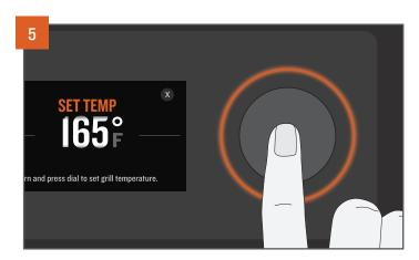
Press the center of the selection dial to select that temperature.
