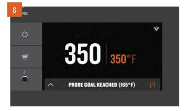
A tone will sound when your protein reaches the set alarm temperature. If using the Traeger app, you will also receive a push notification on your connected smart device.
