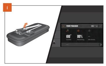
See "Cooking on Your Traeger" on page 20 to turn on the grill. Once the grill is on, remove a charged Traeger® Bluetooth Probe one at a time from the charging dock and the controller will automatically recognize any previously paired probe. A probe widget will appear within the Traeger Dashboard where you can find additional information on probe status and shortcuts for setting probe goal alarms.
